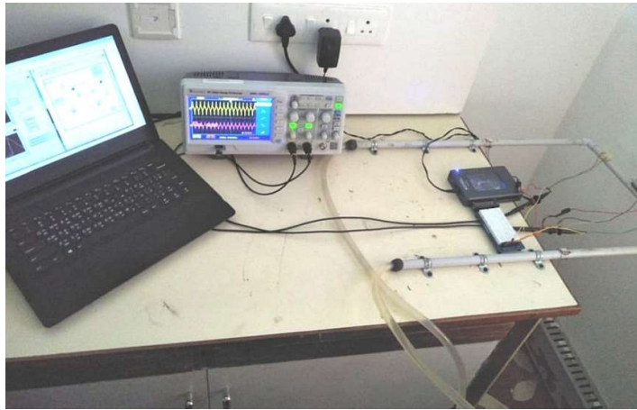
FIG-6 EXPERIMENT SETUP OF U-TUBE CORIOLIS MASS FLOW METER
